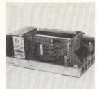
Electronic heart of the Computer Transceiver Systems, Inc Execuporta portable data terminal housed in a luggage-type case for remote communications with a central computer using a telephone—is a 6 x 10" LSI board. A high density, 2-sided circuit with plated-through holes, it serves to interconnect all major parts of the terminal, including keyboard, printer, and power supply. Logic functions in-
