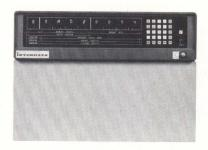
Interdata's 7/32 minicomputer is an economical 32-bit machine with a main memory expandable up to a directly-addressable million bytes of 750 ns core.
