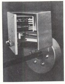
Direct digital control valve is combined with microprocessor for use in small- to medium-sized control systems where only a few pressures, temperatures, or liquid levels are being monitored and controlled continuously
