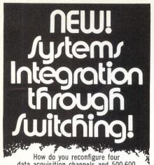
data acquisition channels and 500-600 transducer leads from each of eight test stations — frequently, reliably, quickly, without distorting low level analog signals? Easy. Integrate your system with a matrix switch using 60-circuit T-Bar "Pluggables" that mate directly with wrappable connectors.
