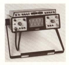
to be the only instrument that provides digital multimeter (DMM), frequency counter, and oscilloscope in one convenient package. Each sub-instrument with its own dedicated display can be used simultaneously with the others or as a complement, or they may be used independently at the same time. Package size is 3% x 8% x 12%, and weight is 10 lb.
