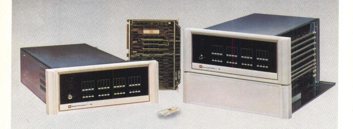
Introducing the 9900 Microprocessor and 990 Series Micro/Minicomputers
